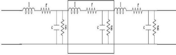
Fig. 1 Transmission line equivalent circuit
