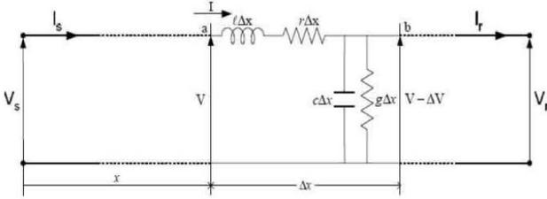
Fig. 2 Small section of a transmission line
