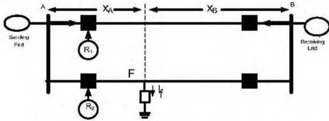
Fig. 5 Power system with a double circuit transmission line
