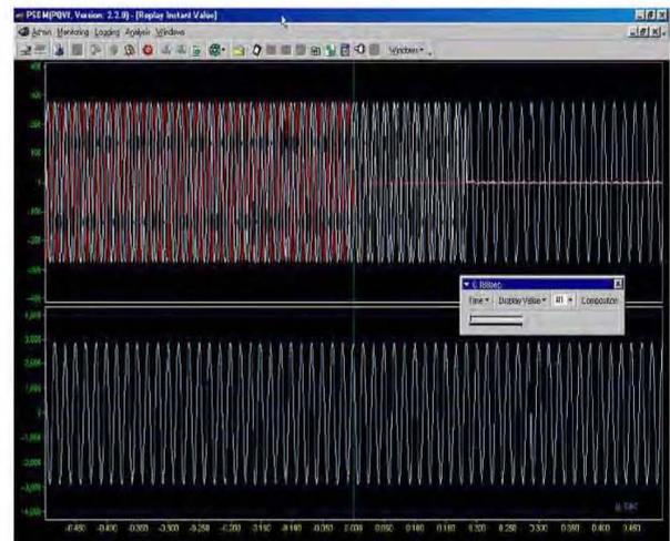
Fig. 7 Arrival of travelling waves at the fault recorder
