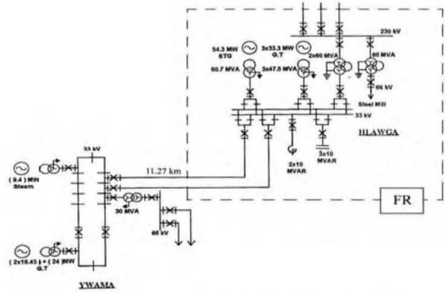
Fig. 6 One line diagram of Hlawga substation with fault recorder
