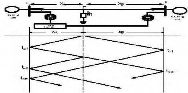
Fig. 4 Travelling waves on a single circuit transmission line
